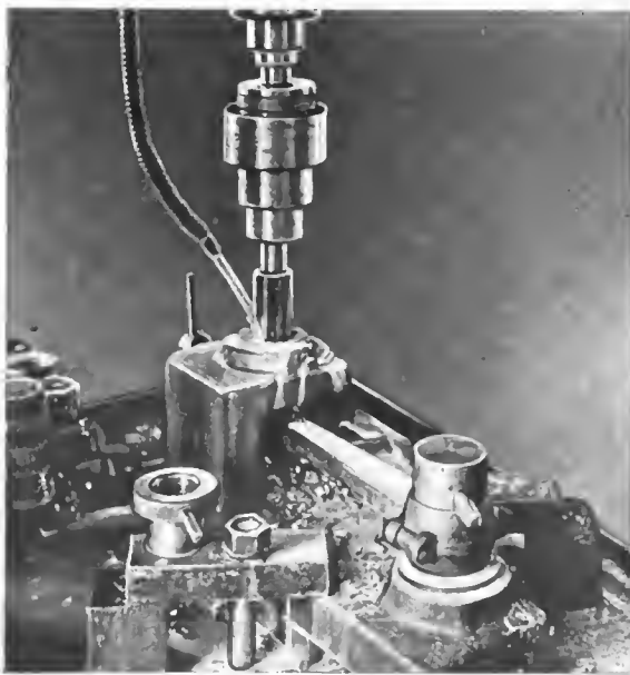
B—Connecting Rod Mounted in a Fixture on the Platen of a Power Reamer Having the Piston Pin End Reamed to Exact Diameter.
